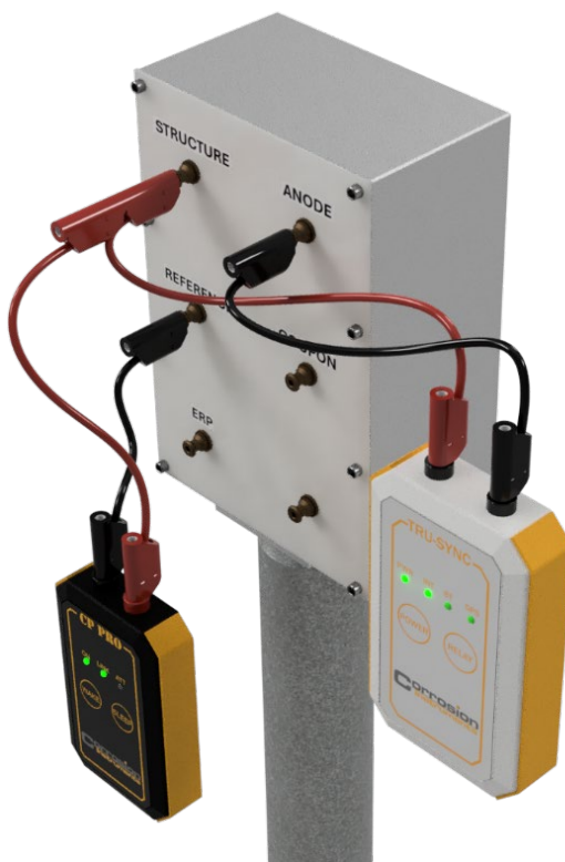
Figure 2 - Illustrates the common configuration where the TRUSync Portable is connected between the Anode and Structure, with a test meter installed between Structure and Reference
